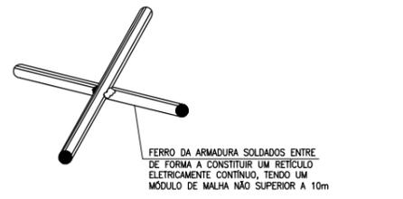
DETALHE DE CONTINUIDADE ELÉTRICA 1 SEM ESCALA
